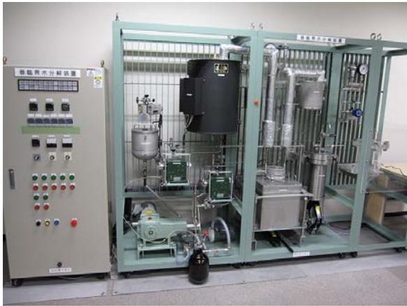
Figure 3 Bench-scale plant for hydrolysis of paper sludge
