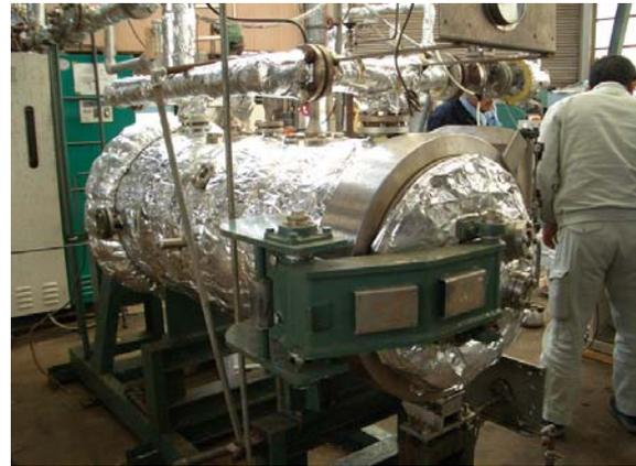
Figure 4 Pilot-scale plant for production of powder fuel
